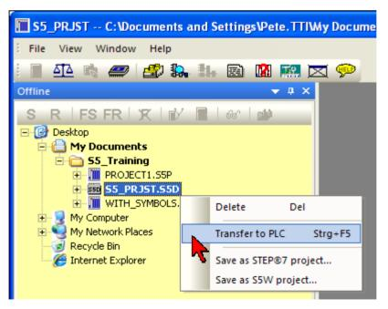
The PLC project, with all the PLC Blocks, is transferred to the connected PLC.
