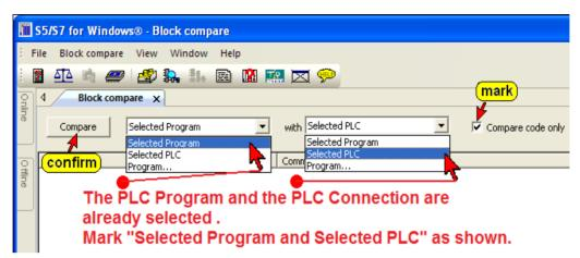
When comparing a PLC Program on the PC with the Program executed on the PLC, only the code is relevant. Mark "Compare code only". To start the comparison confirm by clicking the "Compare" button.
