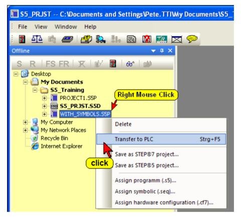
The PLC project, with all the PLC Blocks, is transferred to the connected PLC.
