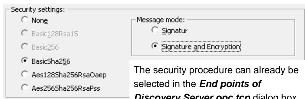
If a security procedure is selected, certificates must be exchanged between the **IBH OPC Editor** and the **OPC UA Server** (IBH Link UA).
