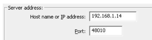
If there is no DNS server, the absolute IP address of the **IBH Link UA** (192.168.1.14) must be entered with the port (48010).
