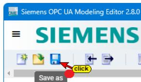
All required specifications have been completed for the example. By clicking the **Save As** symbol, the configuration is saved as an **.xml** file. The **.xml** file (**SiOME Nodeset Manual Example.xml**) is ready to be read into the IBH UA Editor as a **NodeSet**.
