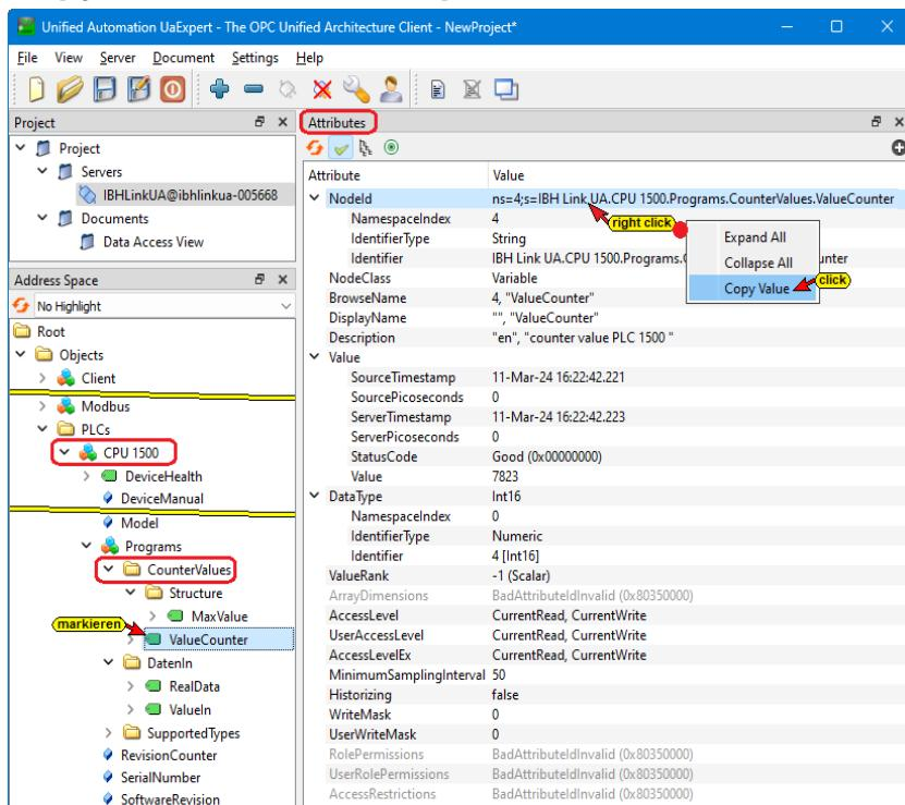
If the OPC variable configuration created in the OPC UA Editor was transferred to the IBH Link UA, the **Nodeld** of an OPC variable can be copied in the window of the **UaExpert** program. If a variable is marked in the **AddressSpace** window, its **Nodeld** can be copied in the **Attributes** window.
