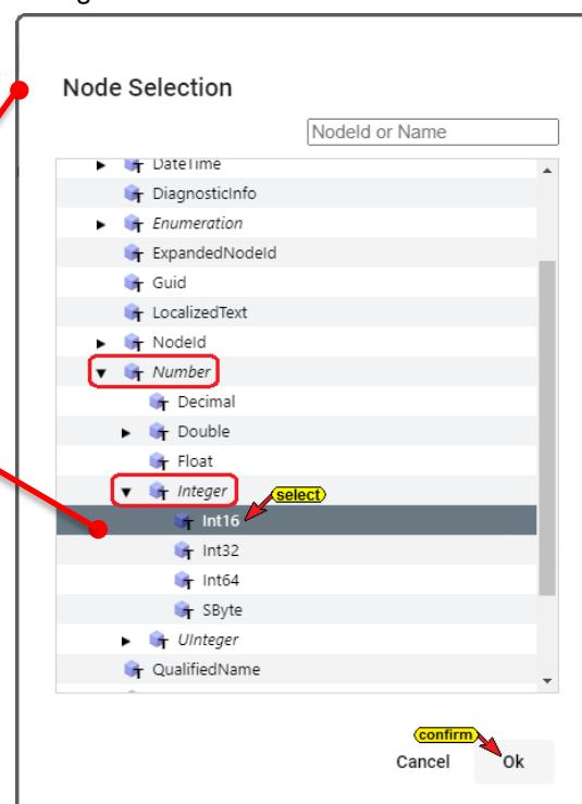
In the same way, create the variable **OutRes** with the data format **Int16**. The variable **InVar** and **OutVar** are created with the data format **Float**.
