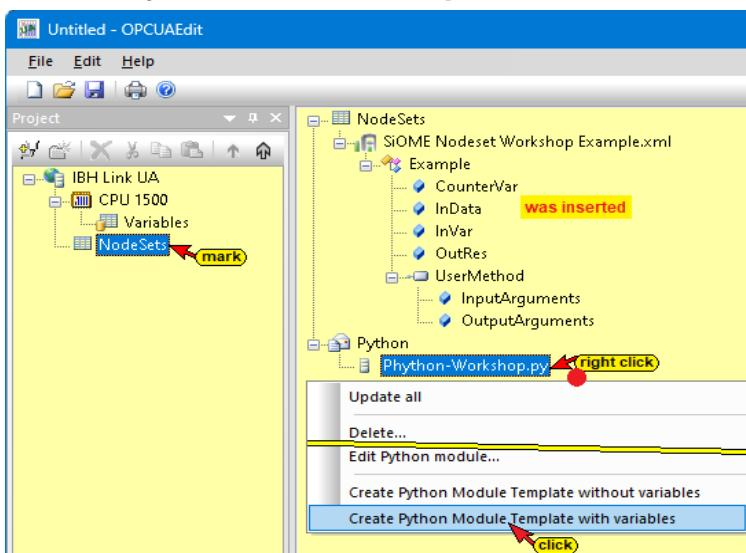
Right-click on **Python-Modul.py** and a click on the **Create Python module template with variables...** command. The configuration is created based on the configuration created in the **SiOME OPC UA Modeling Editor**.
