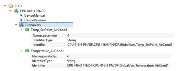
These variables are used as pointers when calling USEND with parameter *SD\_1*.
