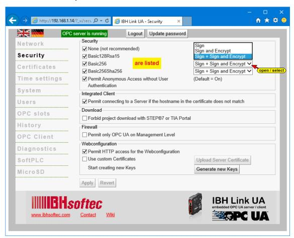
The security configuration of the server is requested by the client via the **SecureChannel** to set up the communication channel. This guarantees the security (confidentiality) and integrity of the transferred messages.
