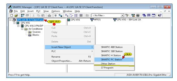
Rename the inserted SIMATIC PC station (1) to IBH Link UA.
