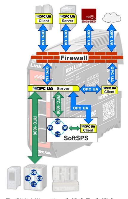
The IBH Link UA contains a SoftPLC. The SoftPLC can read and write variables from the OPC UA server.
