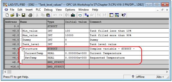
A structure was created in the data block DB2 *Tank\_level\_values*. The DB has been defined in the symbol table.
