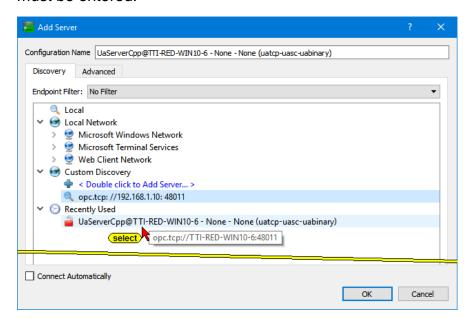
The external OPC Server *UaServerCpp*©<*PC-Name*> provides only the security level *None - None (uatcp-uasc-uabinary).*
