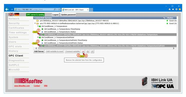
In addition, *CurrentTime* of the external server must be added as a *Read Variable*.
