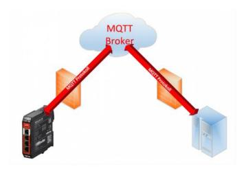
The configuration takes place via an XML file, which is read in via the web interface under "Client". Multiple connections to different MQTT brokers can be made simultaneously.
