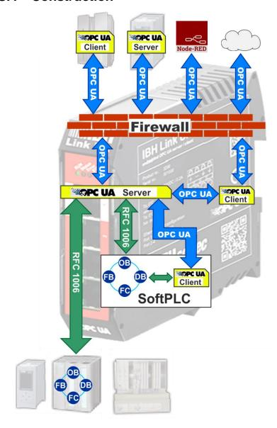
The IBH Link UA is a server / client module. The OPC client function allows data exchange between OPC servers.
