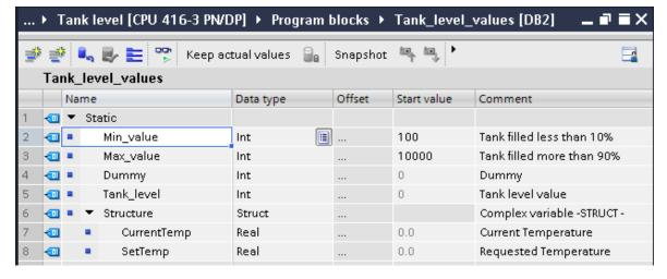
A structure was created in the data block DB2 Tank\_level\_values.
