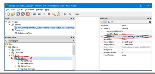
The operands listed in the symbol table, defined as OPC tags, are displayed below *GlobalVars*. Using Drag&Drop they can be pulled into the *Data Access View*.
