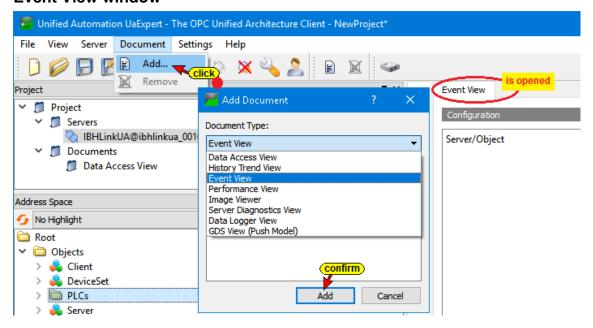
Use Drag&Drop to move the complete PLC – *IBH Link UA SoftPLC [WinAC RTX]* in the *EventView* window. All the alarms coming from the PLC are displayed. It is not possible to select individual alarms.
