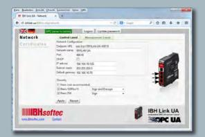
The IBH Link UA is an OPC UA Server/ Client module with integrated firewall for the SIMATIC S5, S7-200, S7-300, S7-400, S7-1200, S7-1500 and LOGO! (Ethernet versions) PLC. It is a compact unit for DIN rail mount with four Ethernet ports and a 24V power supply.
